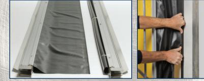
No fabric trimming on side seal panels for projection mount installations. Panels are preinstalled in the door track at the factory. The wall side of the panels are snapped into the wall mounted receiver.
