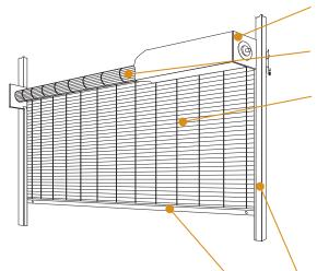
**BRACKETS** - Steel with SpectraShield<sup>®</sup> powder coating in Gray. Bolt to guide assembly and support counter-balance shaft and curtain.
