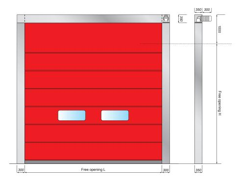
High speed fold up door "VertiGo" - Side Motor
